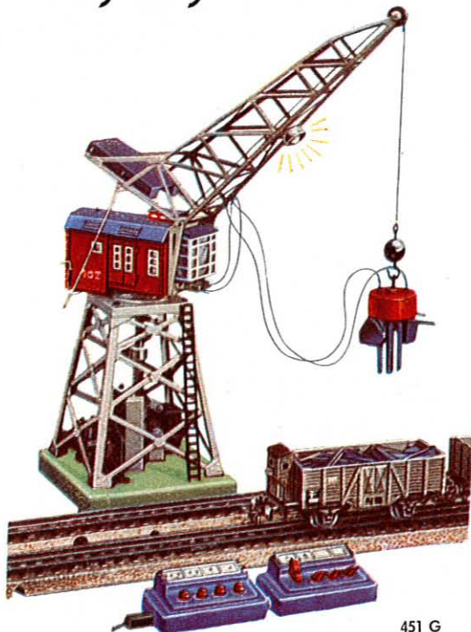
451 G $ 33.— The remote controlled crane with electromagnet • Electrically powered and remote controlled • 2 motors for turning boom and raising or lowering the load • Remote controlled hook and magnet make it possible to transfer metal objects without help from the human hand • Boom may be raised or lowered by manually operated crank • Searchlight on boom and illumination inside cab, may be shut on or off by remote control • Numerous other details • Finely enamelled • Height about 10 1/2 inches • Base plate about 3 1/2 by 3 1/2 inches • With one yard of cable and two control plates for remote control. (Track and rolling stock not included)
