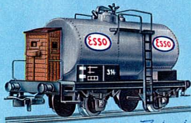
314 E 31-10-93 Tank Wagon with brakesman's cabin · Light grey "ESSO" · Gangway with ladder and fillers · Length about 4 in.
