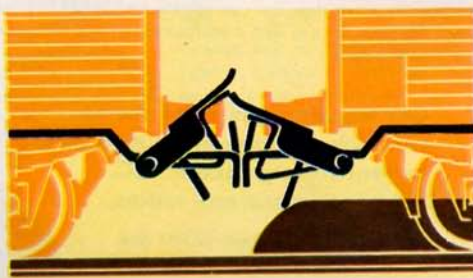
The couplings are uncoupled by raising an actuating ramp between the rails
