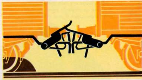
This design of coupling allows the train to be shunted further after the track uncoupler has acted, without the couplings re-engaging
