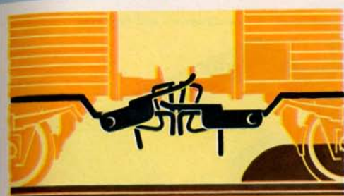
The couplings are uncoupled by raising an actuating ramp between the rails
