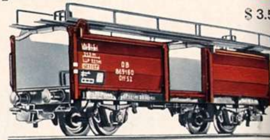
Motor Vehicle Transporter with loading ramp · Not loaded · Brown, with black ramp · 4½ in. long · (On the German Federal Railways two of these transporters are always used together as a unit which is then described as the Off 52 Type)
