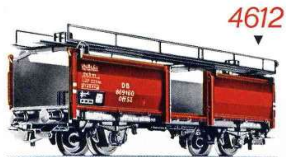
4612 AUTOMOBILE TRANSPORTER • Not loaded • Brown • Black loading Ramp • 4 1/2 in. long • (On the German Federal Railways these cars are used in pairs and the unit is then designated Type Off 52)
