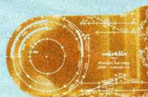
0206 Track planning stencil for Märklin HO gauge metal track sections of 5100/5200 series · Track sections, turnouts, crossings etc. are marked out on the stencil in 1:10 scale, and with a sharp pencil they can easily be reproduced on paper
